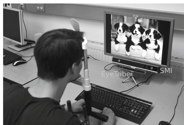
Fig. 2 Setup of experiment with the SMI-RED 120-Hz eye tracker positioned above the EyeTribe eye tracker. Note that the images presented on the screen were actually in gray scale
